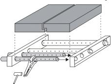
Note: When cleaning the chimney reverse the above procedures, removing the air tube and baffle bricks and then replace them when cleaning is completed.
